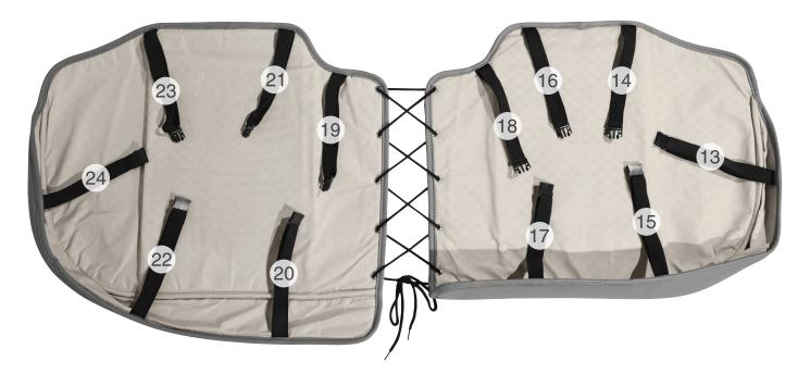
⑦ Tighten the string in the center and tie a knot when the covers are properly positioned.
