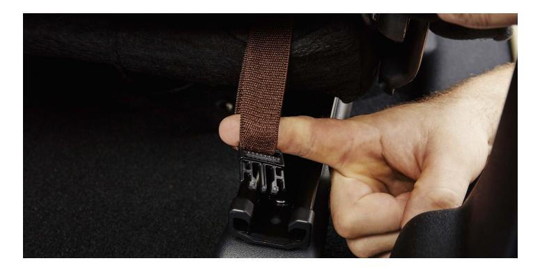
Lay the seat cover bottom so the seat cover lip wraps around the base of the car seat. Slide the inner straps (5 & 6) through the separation between the upper and lower sections of the front seat. Now take the straps on the outer side (7 & 8) of the cover and connect them to the corresponding inner straps after stretching them around the hinges of the front seat.
