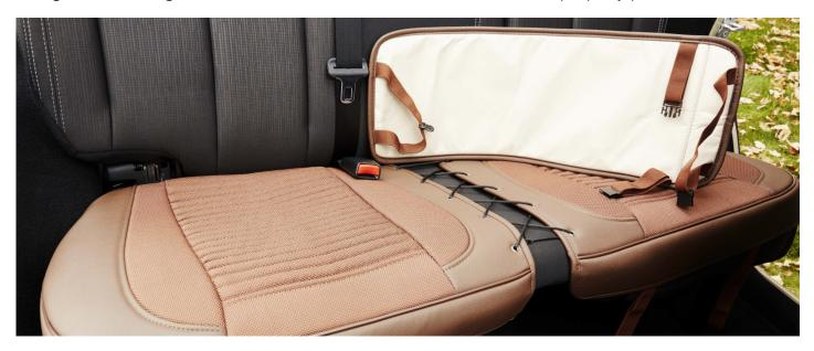
⑧ Using the center seat overlay with straps, cover the string and secure the straps (25 connects to 26 and 27 connects to 28) after wrapping them around the rear seat base. Strap 27 and 28 may not be necessary for your vehicle. You can connect them and hide them under the center overlay.
