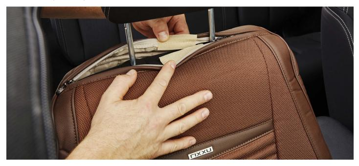
① Slide the straps (1 & 2) on the lower inner back side of the cover through the separation between the upper and lower sections of the front seat. Now take the straps on the outer back (3 & 4) side of the cover and connect them to the corresponding inner straps (2 & 3 connect, 1 & 4 connect) after stretching them around the hinges at the base of the upper front seat section.
