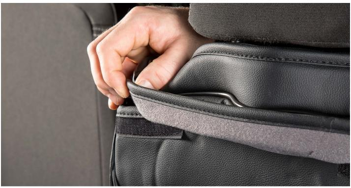
Pull sides firmly on the left and right side of the seat to attach the hook and loop fastener to the front (hook and loop fastener compatible) portion of the seat cover.
