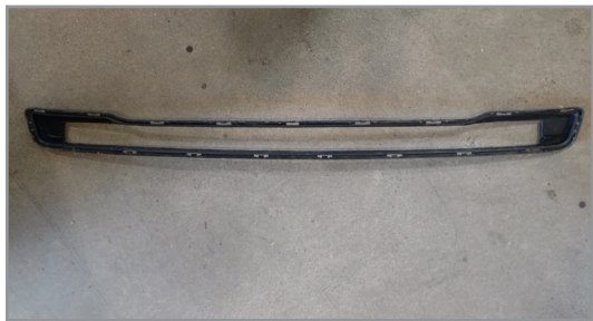
Finish Trimming by Cutting Just Inside the Horizontal Bezels (40" Width Shown)
