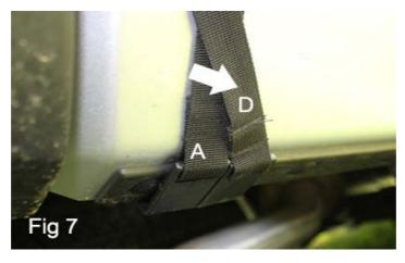
Adjust all straps so that the inner flap seam is even with the top of the bed rail (Fig 8 and Fig 9).
