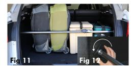
**7-**Rotate the rubber pads (Fig 12), if necessary, and move the handle back and forth until the Cargo Bar tightens snugly against the walls of the SUV cargo area.
