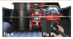
**6-**Rotate the rubber pads (Fig 5), if necessary, and move the handle back and forth until the Cargo Bar tightens snugly against the walls of the truck bed.
