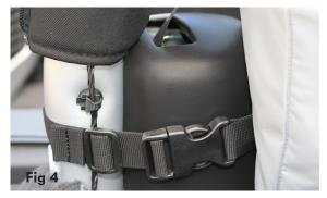
**3-**Buckle the E strap over the rear seat belt holder, without twisting the strap (Fig 3 and Fig 5).
