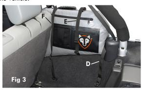
**2-**Buckle the D strap around the base of the rear angled roll bar, without twisting the strap (Fig 3 and Fig 4).
