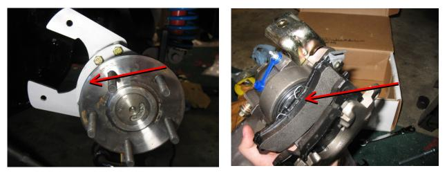
Slide the caliper into position, have the brake pads go on each side of the rotor and the two mounting holes on the caliper will match up with the two holes in Bracket #2.
