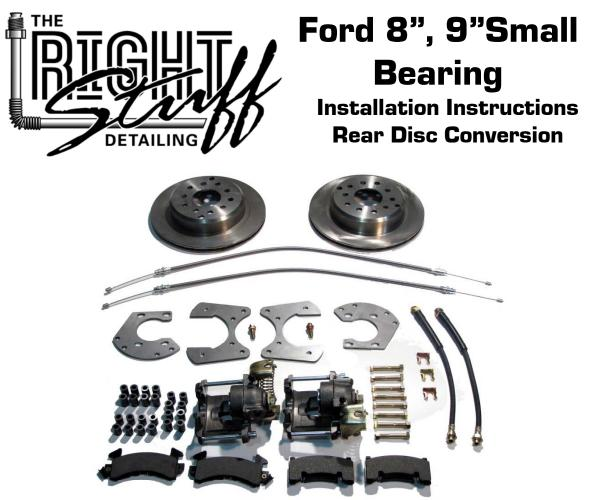
This kit is for Ford 9" rear axles with the small (2.835") style bearing and Ford 8" rear ends. This kit is designed to work with axles with either GM 5 x 4.75 Bolt Pattern and 7/16" wheel studs or Ford 5 x 4.5 Bolt Pattern and  $\frac{1}{2}$ " wheel studs. Rotor center measures 2.78".
