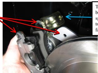
The zinc plated bracket with spring attached to it needs to face upwards.
