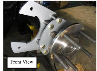
Slide the rotor onto the studs. The rotors are drilled for both Ford and Chevy bolt pattern. Hand thread two lug nuts to seat the rotor in place for test fitting.
