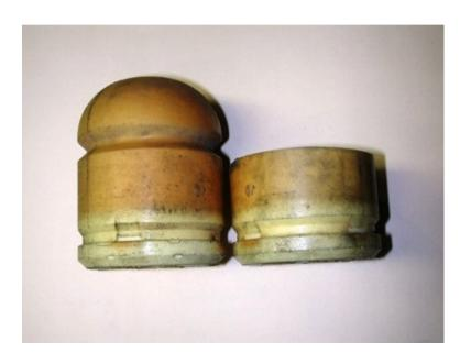
3. Remove the bump stop from the frame and cut the upper convolution off, then reinstall back onto the frame. This will allow for maximum drop.
