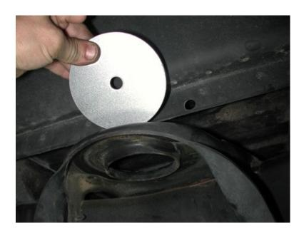
6. Place the 4" washer on top of the upper coil spring mount.
