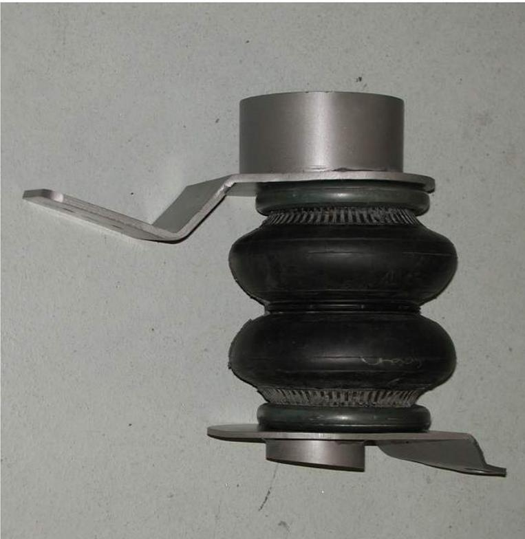
4. Assemble the upper and lower brackets onto the airspring as shown to the left. This is the driver side assembly as viewed from the front. Be sure to install the airline fitting into the airspring and position it so the airline has a clear exit to the side of the upper cup.
