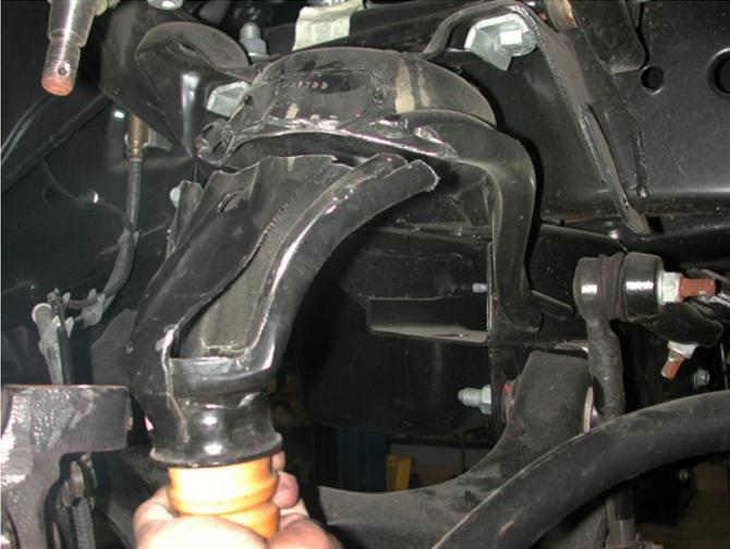
3. The 1 ton Dodge has a large protrusion that extends from the upper coil spring pocket that supports the compression bump stop. This protrusion will be trimmed off. This can be accomplished with a cutoff wheel, torch, or a sawzall.
