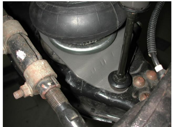
7. This photo shows how the lower bracket is positioned by the oem sway bar mount.
