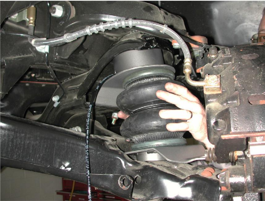
5. Insert airline into fitting and install the airspring and bracket assembly into the front suspension as shown. Note that the upper bracket "tongue" will be inside the crossmember as shown below. The lower bracket will be positioned by the oem sway bar hole in the lower control arm.
