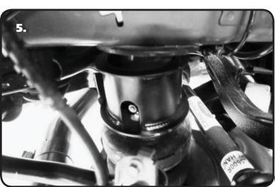
**5.** Install the Air Spring/Upper Cup Assembly into the OEM coil spring location. The top of the Upper Cup will sit in the OEM coil spring location. Clock the fitting to the front of the car, but be sure you have access to it to install the air line. The bottom of the Air Spring will sit on top of the Lower Cup Bracket.
