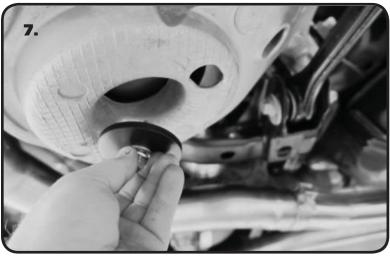
7. Move the Air Spring around until the threaded hole lines up with the holes in the Lower Cup Bracket. Insert the Clamping Plate into the coil spring centering ring hole in the bottom of the lower control arm, threading the 3/8"-16 Hex Bolt into the bottom of the Air Spring. Hold the Air Spring to keep the fitting hole in the correct location and Torque the 3/8" Hex Bolt to 15-20 ftlbs.
