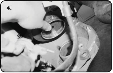
**4.** Install the Lower Cup Bracket into the OEM coil spring pocket of the control arm. The Cup Bracket is installed with the bottom ring located around the coil spring centering ring on the control arm.
