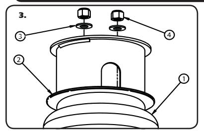
**3.** Thread a 90 Degree Fitting into the Air Spring with Thread Sealant applied to the threads. Place the Upper Cup Bracket(2) on to the top of the Air Spring(1). Next, install a 3/8" Flat Washer(3) on each threaded stud, followed by a 3/8"-16" Nylok Nut(4). Torque Nuts to 15-20ftlbs.
