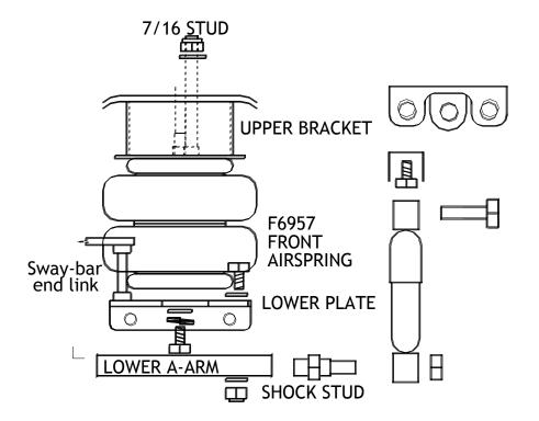
4. When the attachment holes are finished, assemble the airsprings onto their brackets and install the airline fitting [see sketch to the left]. Be sure to use Teflon tape or paste to prevent air leaks. 5. Install the airspring/bracket assembly into the oem coilspring location. A supplied threaded stud, stepped washer, and nyloc nut will attach the upper cup and supplied bolts will fasten the lower control arm plate.
