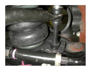
3. Fit the lower airspring plate into the lower control arm. This plate will be positioned by the oem swaybar hole. The remaining attachment holes will need to be drilled into the control arm using the plate as a template.
