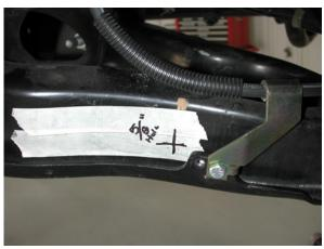
7. The bottom of the shock is attached to the rear of the lower control arm slightly inboard of the bracket tab shown to the left. A 5/8" hole is needed to install the provided shock stud. Check you tire clearance closely before selecting the final location for this stud. After the stud and shock are installed, the upper bracket may be final tightened.
