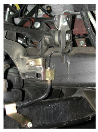
6. Install the upper shock mount and brace assembly onto the rear upper control frame bracket. Do not tighten the shock bracket bolt until the shocks are actually installed to set the final angle of that bracket.
