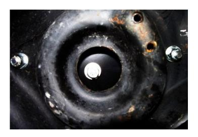
9. Fasten the air spring to the lower plate using a 3/8" x 1" bolt, lock washer and flat washer.
