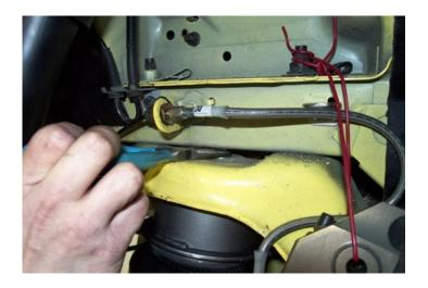
8. Fasten the air spring assembly to the frame in place of the coil spring, using a 7/16" nut and flat washer. The air fitting access should face toward the engine. It may be easier to use a needle nose pliers to get the nut started on the stud.
