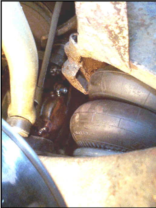
Trim the outer pocket where the bumpstop contact bracket would rub on the airspring
