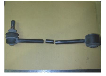
10. For necessary clearance and optimum effectiveness the sway bar end link must be shortened by approx. 1" so that it is 7 <sup>3</sup>/<sub>4</sub>" long from center eye to center eye. This 1" section will have to be cut from the center of the link and then welded back together.
