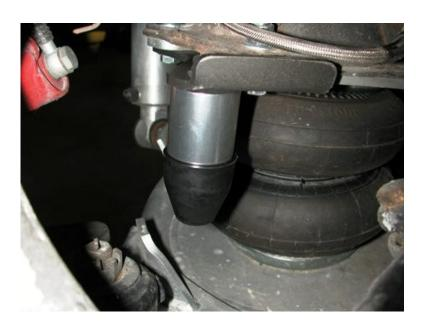
**Note**: It is acceptable to let the suspension bottom on the air spring. However, if your tire hits the inner fender well before the air spring bottoms out, this bump stop must be installed.
