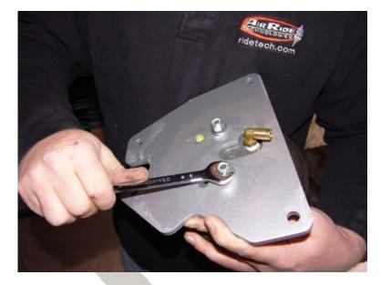
2. Apply thread sealant to the air fitting and thread into the air spring.
