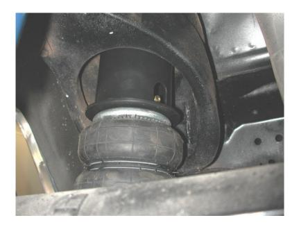
5. Raise the assembly into the coil spring pocket with the all thread sticking through the upper washer. Secure the assembly with a 7/16" Nylok nut and flat washer.
