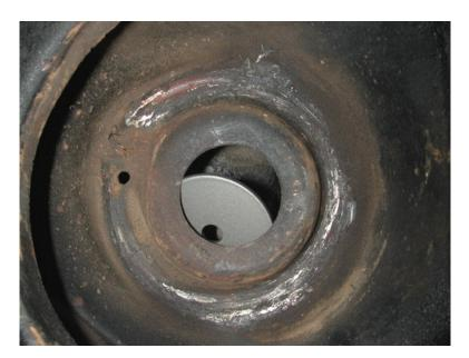
4. Place the upper washer on top of the coil spring pocket.
