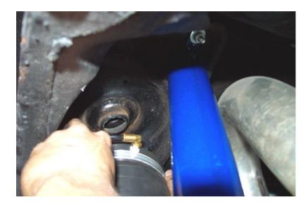
5. Place the 4" diameter washer on top of the frame, above the coil spring pocket. Raise the air spring up to the spring pocket with the pin sticking through the washer. Secure with the large cotter key.
