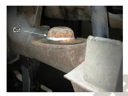
3. To allow the air spring to sit flat on top of the axle mount, the coil spring retainer must be cut down to about 1/4" tall. Leave just enough of this retainer to locate the air spring roll plate, but make sure it is short enough not to contact the air spring piston.
