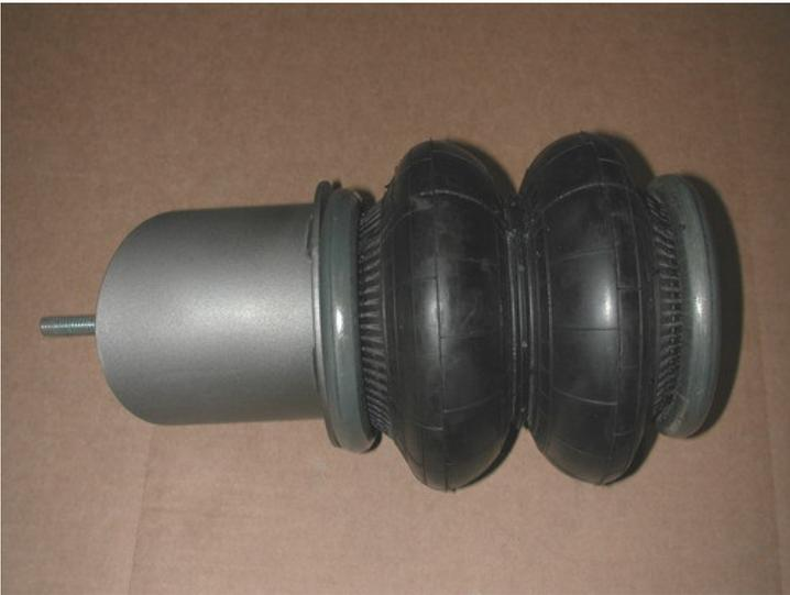
3. Insert air fitting into air spring using tread sealant. Place the upper cup onto the studs on the air spring and tighten using two 3/8" nyloc and flat washers. Thread the 6" stud into nut in bottom of air spring cup.
