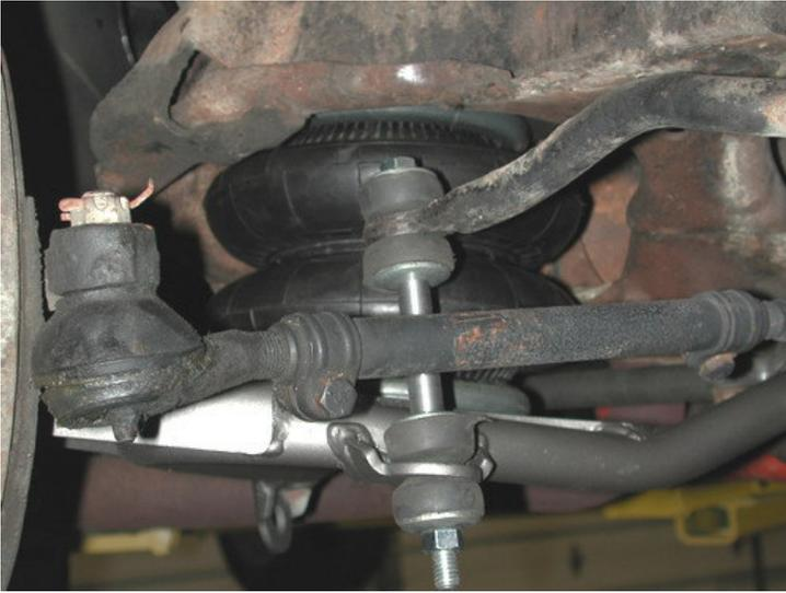
6. The sway bar end link must be shortened to 2" tall optimize clearance and alignment. Use the shorter 3/8" x 6 1/2" bolt supplied.
