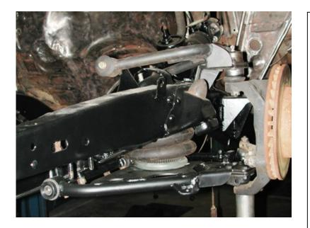
7. Bolt the lower air spring plate to the lower arm using  $3/8" \times 1"$  bolts, flat washers and Nylok nuts. The two outer holes will align with the factory bump stop holes. The inner two holes must be drilled. Bolt the air spring to the lower plate using  $3/8" \times 3/4"$  bolts, flat washers and lock washers.
