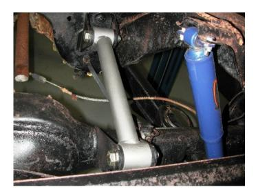
1. Attach shock T-Bar to frame using 3/8" x 1 1/4" bolts, Nylok nuts and flat washers.
