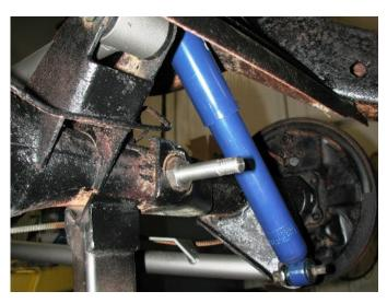
2. Attach the bottom of the shock to factory shock stud using the ½" Nylok nut & flat washer supplied. Install one aluminum spacer on each side of the bearing.
