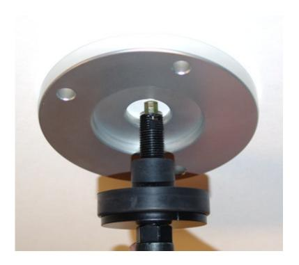
3. Bolt the aluminum upper plate to the car in place of the factory rubber mount using the 3/8" x 1 1/4" bolts, flat washer and Nylok nuts.
