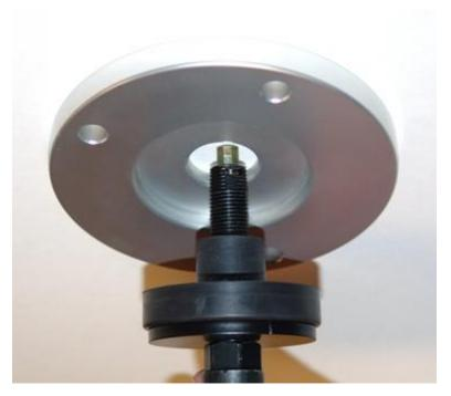
4. Bolt the aluminum upper plate to the car in place of the factory rubber mount using the  $3/8^{\circ} \times 1 \frac{1}{4}^{\circ}$  bolts, flat washer and Nylok nuts.
