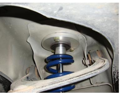
6. From the engine bay, place the other rubber bushing over the stud, then another steel plate. Secure the assembly with a 9/16" SAE Nylok Jam nut. **Note:** Some cars may have a plastic cover in the engine bay that may need to be clearance for the adjustment knob.
