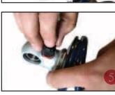
Install upper spring mount retainer clip (90002057) into the groove on the upper eyelet as seen in figure 5. Then reinstall adjuster to complete assembly.
