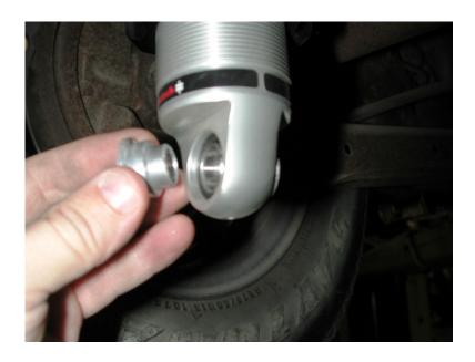
8. Install the aluminum spacers into the upper and lower eyes of the shock.
