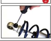
Before the upper spring mount can be installed screw the adjuster knob on the upper eye mount to the firmest setting (clockwise) as seen in figure 3.
