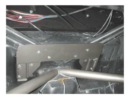
6. The inner support plate will bolt to the floor pan on the inside of the car using six 3/8" x 1" bolts, Nyloks and flat washers. The remaining 4 holes will need to be drill and will use 3/8" x 2 1/4" bolts, Nyloks and flat washers.
