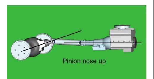
13. How do you set the pinion angle? On a singlepiece shaft you want to set it up where a line drawn through the center of the engine crankshaft or output shaft of the transmission and a line drawn through the center of the pinion are parallel to each other but not the same line.
