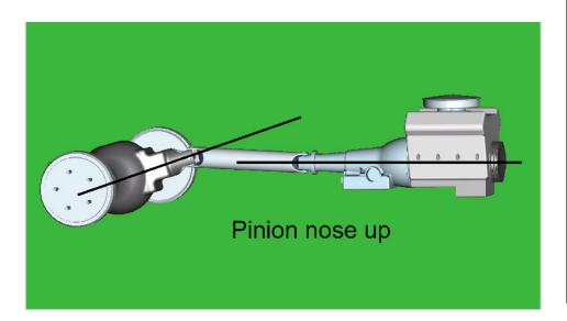
14. How do you set the pinion angle? On a single-piece shaft you want to set it up where a line drawn through the center of the engine crankshaft or output shaft of the transmission and a line drawn through the center of the pinion are parallel to each other but not the same line.
