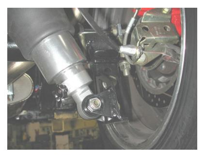
7. Bolt the lower axle bracket to the leaf spring pad using the 9/16" U-bolts and hardware supplied. Bolt the lower Shockwave mount to the axle bracket using the 5/8" x 1 1/4" bolts and Nylok nut.
