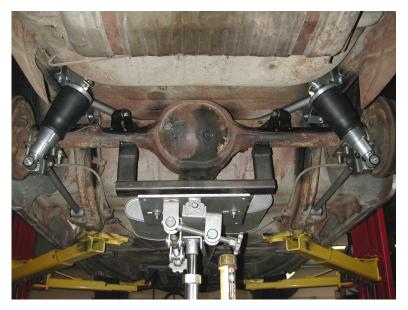
14. Bolt the axle tabs to the upper bar using a 5/8" x 2 3/4" bolt and nyloc as shown in the picture. The upper bar should measure 12" C-C.
