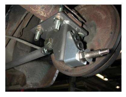
5. Slide the cradle into place with the upper Shockwave mount toward the rear of the vehicle.
