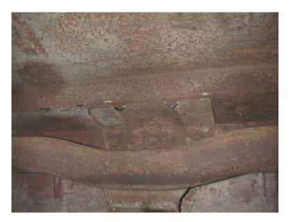
4. You must also trim these grooves in the pan at a 45 deg. angle to allow the upper cradle assemble to slide into place. They are located just in front of the axle above the crossmember.
