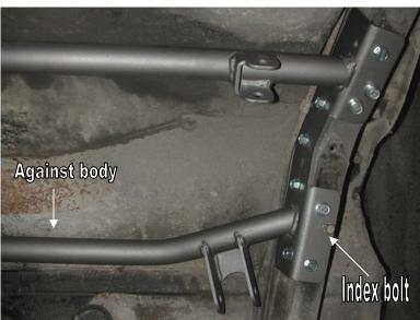
3. A series of self-tapping 3/8" bolts are used to hold the cradle in place. First drill the holes with a 5/16" bit and then thread the bolts into the frame.
