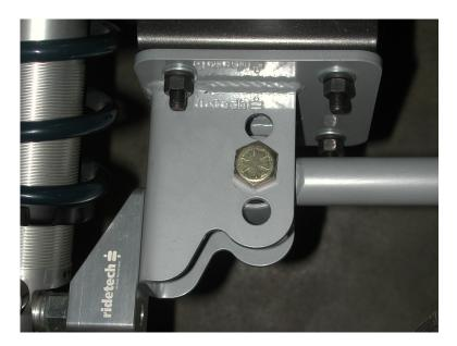
4. The two forward tabs grab the pinch weld and have a backer plate on the inside of the car under the back seat. These are attached using (6) 3/8" x 1 1/4" bolts washers and Nylok nuts.
