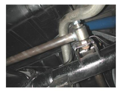
1. Replace the factory panhard bar with the new one using the new stud and hardware supplied. The rubber rod end will be attached to the axle.
