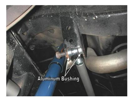
2. The Heim end will attach to the frame using the 9/16" x 3" bolt and Nylok nut. Two aluminum T-bushings need to be installed on each side of the Heim end.
