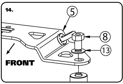
**3.** Sit the Bracket[5] on the Spacer with the holes centered over the Seat Studs. Center the Spacers and Bracket on the Studs. Install a 1/2" Flatwasher on each of the Shoulder Nut[8]. Thread the Nuts on the Studs with the Hex up. The Shank side of the Nut will Thread onto the Studs with the Shank going through the Bracket and Spacer. Tighten Both Nuts.
