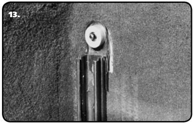
**2.** Install a Lap Belt Bracket Spacer[7] on each Seat Track Stud sticking up. Center the Spacer on the Stud.
