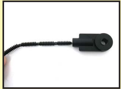
3- After getting the linkage cut to length and shaped, line up the end with the end link.
