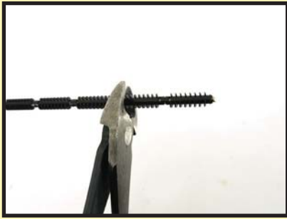
1- The linkage rod can be cut to length using side cuts.
