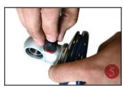
Once the knob is removed Slide the Derlin washer over the spring, Next slide the upper spring mount (90002222) over eyelet as seen in figure 4.
