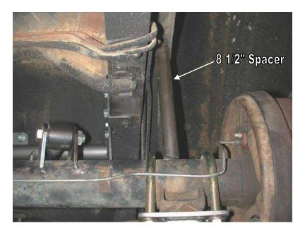
7. Using the supplied U-bolts, fasten the lower axle bracket to the factory leaf spring pad.
