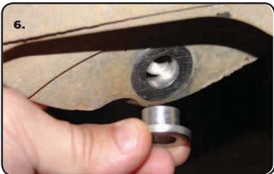
**6.** Insert the supplied T-Bushings into the OEM Control Arm. The T-bushings are installed on the outside of the OEM Control Arm.
