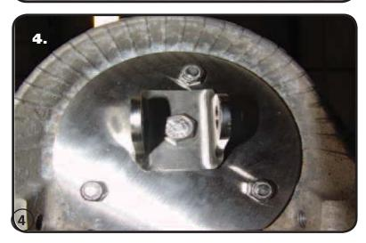
**4.** Install the upper mount into the crossmember using (3) 5/16" x 1 1/2" Hex Bolts, (3) 5/16" SAE Flatwashers, & (3) 5/16" Nylok Nuts. Position the Straight edge of the Mount facing the Engine Compartment. Tighten the mounting hardware.
