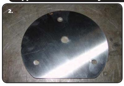
**2.** Both sides of the suspension use the same Upper Mounting Plate. Both Upper Mounting Plates and Shock Mounts are assembly identically to each other. Figure "2" shows the bottom side of the Mounting Plate.
