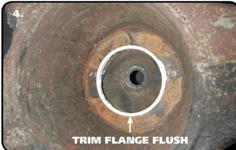
4. Trim the coil spring location ring flush to prevent the ring from hitting the top of the ShockWave Air Spring. A die grinder with a cutoff wheels works well here.
