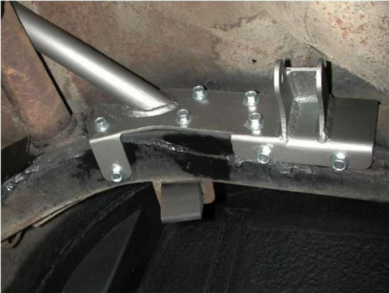
5. Slide the cradle into place with the upper Shockwave mount toward the rear of the vehicle.
