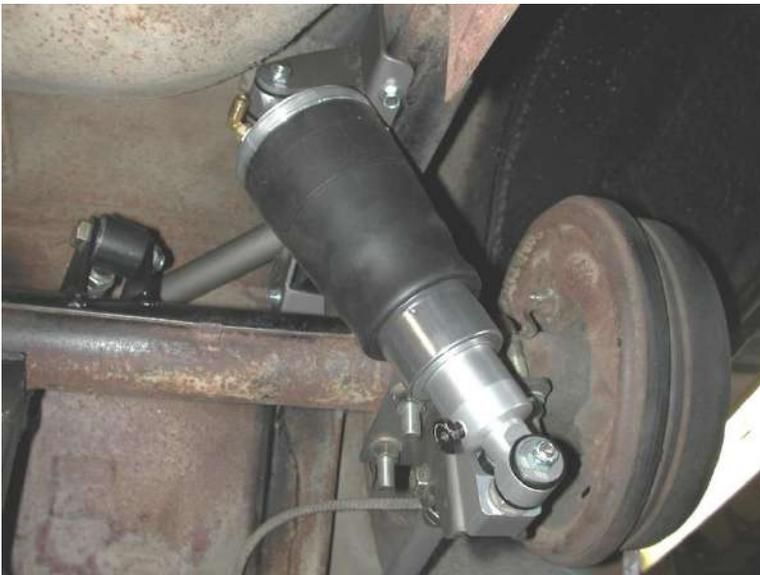
16. This must all be set at **ride height**, which will occur with 14.5" from c-c on the Shockwave mounts. As you can see in the above picture, we have tack welded a 5" long spacer between the axle and frame to maintain ride height, axle center, and pinion angle while welding in the tabs.
