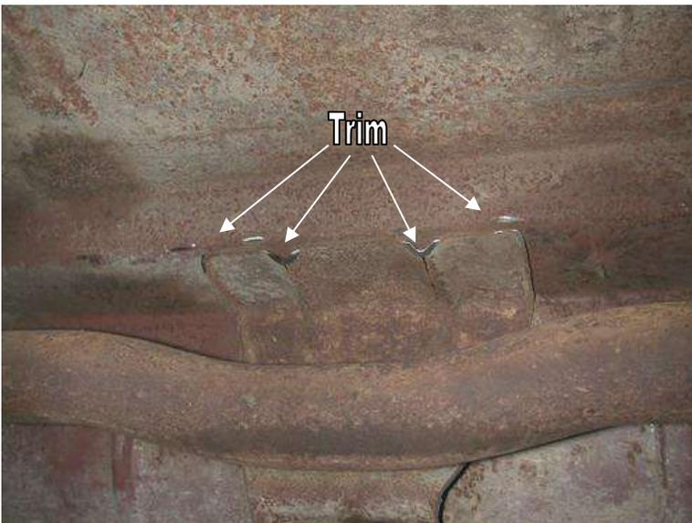
4. You must also trim these grooves in the pan at a 45 deg. angle to allow the upper cradle assemble to slide into place. They are located just in front of the axle above the crossmember.
