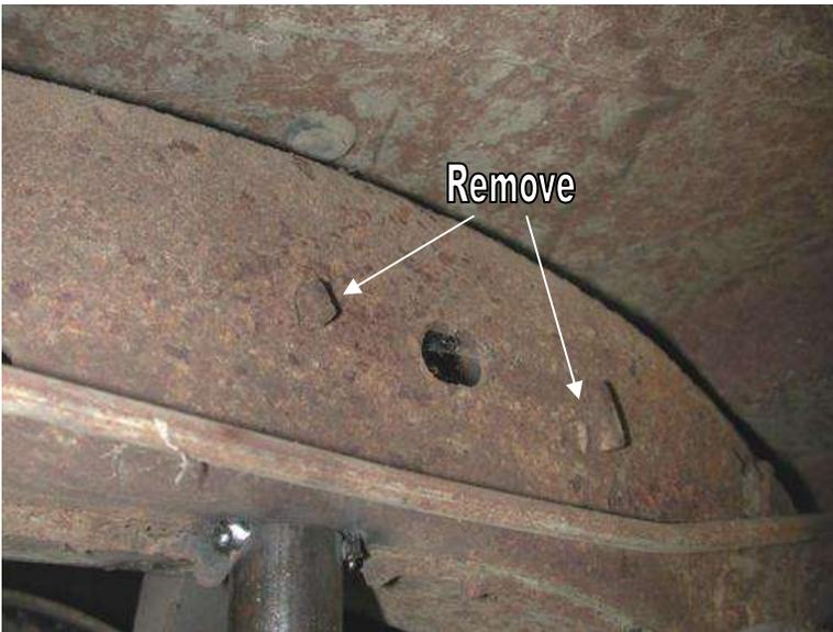
3. On the inside of the frame rail there are two tabs that must be ground smooth.
