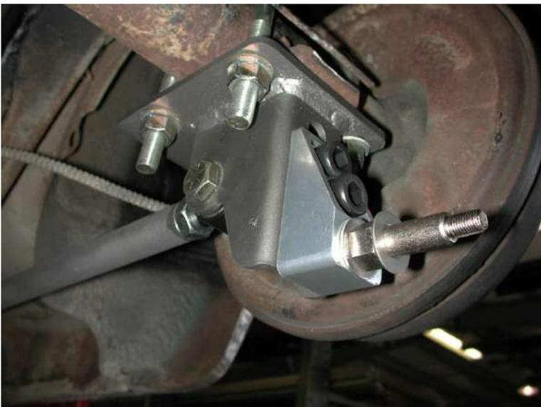
9. Secure the axle mount to the leaf spring pad using the supplied U-bolts. There is an aluminum bushing that will slide over the alignment pin.
