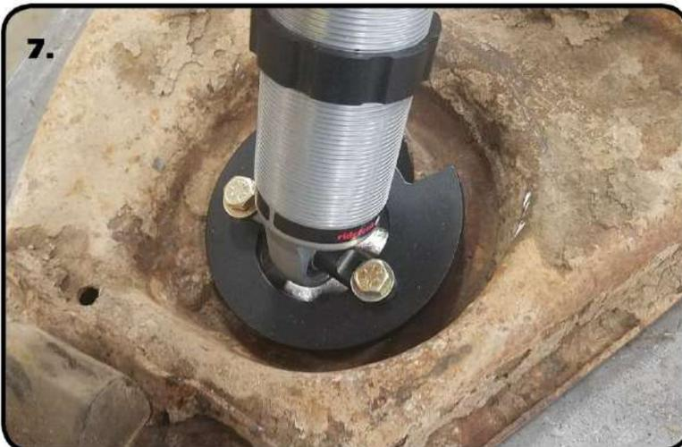
**7. INSTALL THE LOWER CONTROL ARM REINFORCEMENT PLATE.** Refer to **Image 7** for positioning of the plate. Raise the lower arm up to the Shockwave and bolt them together using the 5/16" x 1 1/4" Bolts, Washers, & Nylok Nuts supplied with the ShockWaves. Torque to 17 ftlbs.
