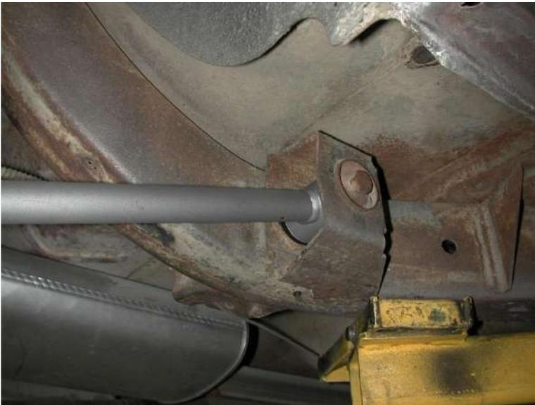
8. Install the Lower Bars. The Front Lower uses the WIDE(70013768) R-Joint Spacers inserted into each side of the R-Joint. The Axle end of the bar gets a NARROW(70013334) R-Joint Spacer inserted into each side of the R-Joint. The bar is attached to the Axle Mount in the **MIDDLE HOLE** using the OEM hardware.
