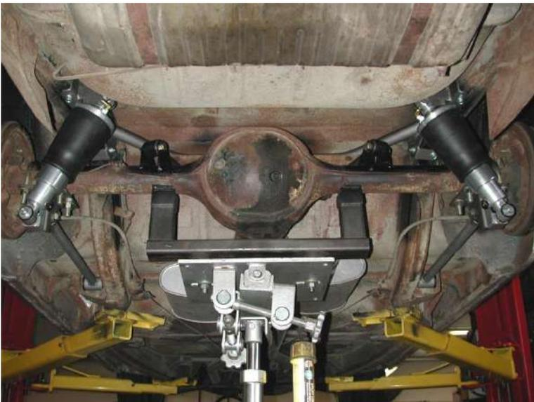
17. Apply thread sealant to the air fitting and screw it into the top of the Shockwave.
