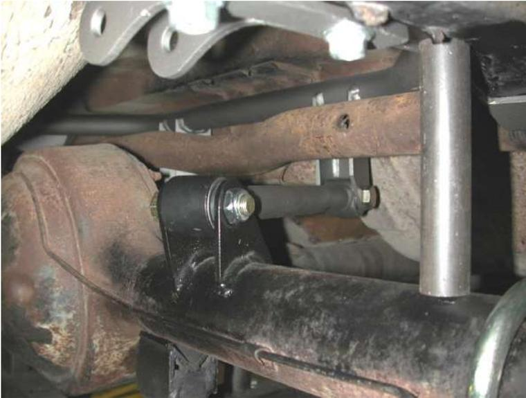
13. Bolt the axle tabs to the upper bar jig using a 5/8" x 2 3/4" bolt and nyloc as shown in the picture. The upper bar should measure 12" C-C.
