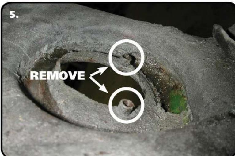
5. The Shockwave trunnion sits on top of the arm as opposed to the factory shock, which bolts to the bottom side of the car. You will have to remove the two OEM nuts that retain the original shock.
