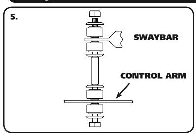
**5.** Install the End Links. Use **(Figure 5)** for proper installation. Tighten the Hex Nut enough to slightly compress the Bushings.
