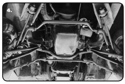
**4.** Slide the SwayBar into position on the Car. The SwayBar Arms will be above the Control Arms. Install a 3/8" Flat Washer on (4) 3/8"-16 x 1" Hex Bolts. A Bolt/Washer will go in each of the 4 mounting holes. With the Bolt/ Washers installed, install a 3/8" Flat Washer on the threads followed by a 3/8"-16 Nylok Nut. Do **NOT** Completely tighten the Hardware. It will be left partially loose until the End Links are installed.
