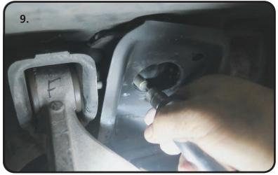
**9.** Clearance the hole if the Mount doesn't sit correctly.
