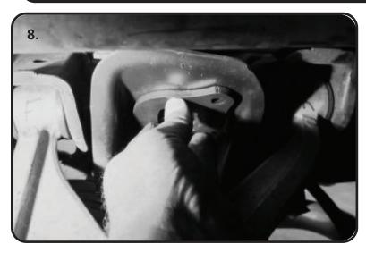
**8.** Insert the 1/2" x 2" Bolt through the holes in the tabs of the Upper Mount. Test fit the Upper Mount to see if any clearancing is necessary. The Mount needs to sit tight against the OEM shock mount with the mounting holes aligned. You may have to clearance the hole for the bolt to fit through it.
