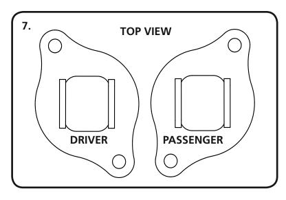
**7.** New Upper Mounts are included to replace the OEM mounts. The Upper Mount will be replaced with mounts included in the Shock Kit. When these mounts are installed correctly, the Upper Mounting Bolt will be PARALLEL with the Lower Mounting Bolt.
