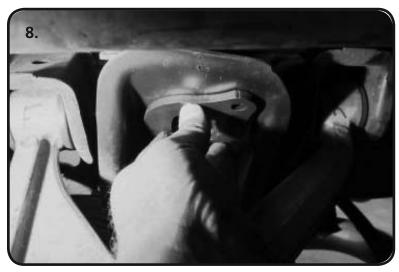
**8.** Insert the 1/2" x 2" Bolt through the holes in the tabs of the Upper Mount. Test fit the Upper Mount to see if any clearancing is necessary. The Mount needs to sit tight against the OEM shock mount with the mounting holes aligned. You may have to clearance the hole for the bolt to fit through it.
