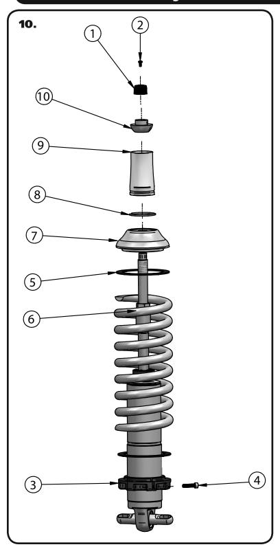
10. To Assemble the CoilOver you need to:a. Remove Screw (2) from center of Adjustment Knob (1) and remove Adjustment Knob.
