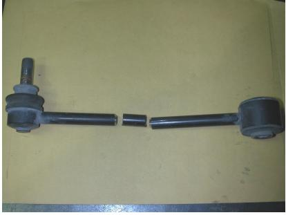
10. For necessary clearance and optimum effectiveness the sway bar end link must be shortened by approx. 1" so that it is 7 3/4" long from center eye to center eye. This 1" section will have to be cut from the center of the link and then welded back together.
