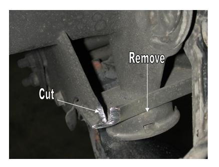
3. To achieve proper clearance of the Shockwave a small corner of the bump stop bracket must be trimmed. This can be done with a cut off wheel.
