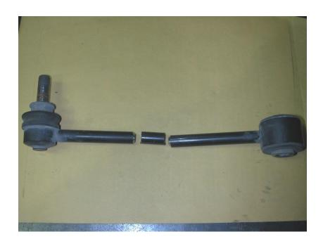
10. For necessary clearance and optimum effectiveness the sway bar end link must be shortened by approx. 1" so that it is 7 ¾" long from center eye to center eye. This 1" section will have to be cut from the center of the link and then welded back together.
