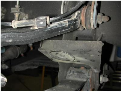
4. To reach maximum drop the bump stop and bump stop cup must be removed. This can be done with a cut off wheel. This picture shows the bump stop bracket after removing the cup.
