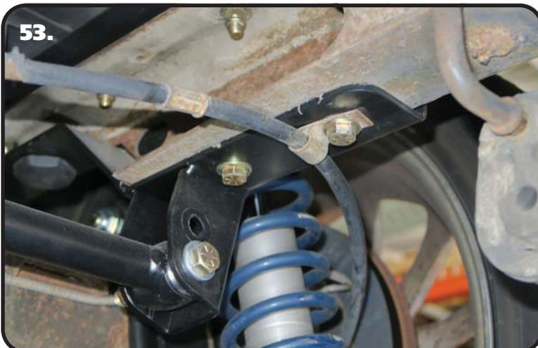
**53.** The passenger emergency brake cable will get attached to the rear bolt of the passenger c-notch. Use the OEM clamp that attached it to the axle housing.
