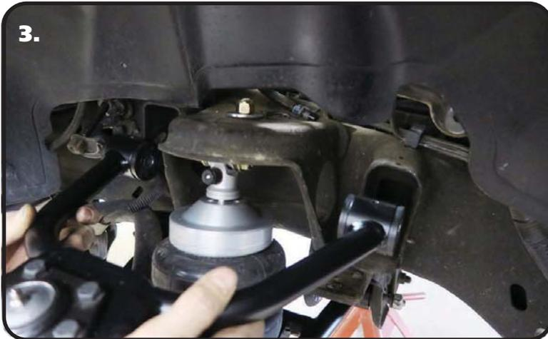
3. The Driver and Passenger Control Arms are identical. Insert the Control Arm into the OEM frame mount with the balljoint stud pointing down. The Gussets of the Balljoint Plate should also point down.
