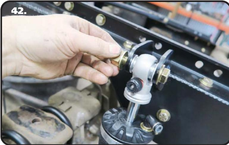
**42.** Insert the 1/2" ID Shock Bearing Spacers into the Bearing of the ShockWave/CoilOver. Install a 1/2" Flat Washer on a 1/2"-13 x 2 3/4" Bolts. Insert the top of the shock into the shock mount on the c-notch with the adjusting knob to the outside. Line up the holes and insert the bolt/washer. Install a 1/2" Flat Washer and 1/2"-13 Nylok Nut on the threads and tighten to 50 ftlbs.
