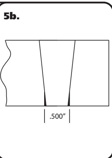
5. Insert the balljoint into the spindle. You will need to clearance the bottom of the taper with a 1/2" Drill bit. Refer to **Images 5a & 5b**. **Image 5b** illustrates the cleared spindle taper. The drawing is exaggerated for illustration purposes.
