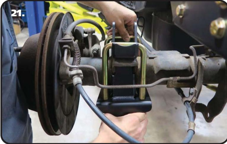
**21.** The axle mounts are the same for driver and passenger sides. Install a supplied 5/8" u-bolt in each side of the upper bar mount. The u-bolts will nest in the slots of the upper mount. Slide an axle mount on the U-bolts with the top tabs inserted into the leaf spring pad.
