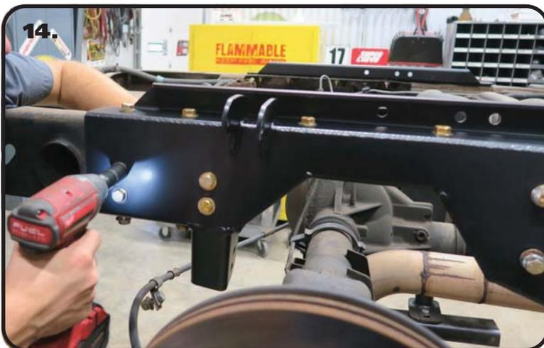
**14.** Tighten all of the c-notch side bolts. Torque to 50 ftlbs.
