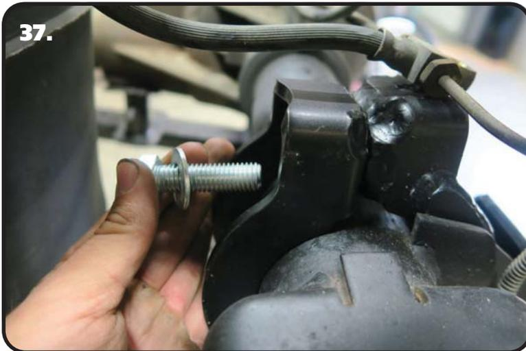
**37.** Install a 1/2" SAE flat washer on each of (2) 1/2"-13 x 1 3/4" bolts. Insert the bolt/washers in the top and bottom mounting holes of the clamp/mount. Install a 1/2" SAE flat washer and 1/2"-13 nylok nut on the threads of each bolt. Torque these bolts to 75 ftlbs. You can now torque the 9/16" hardware that was installed previously. Torque the 9/16" hardware to 110 ftlbs.
