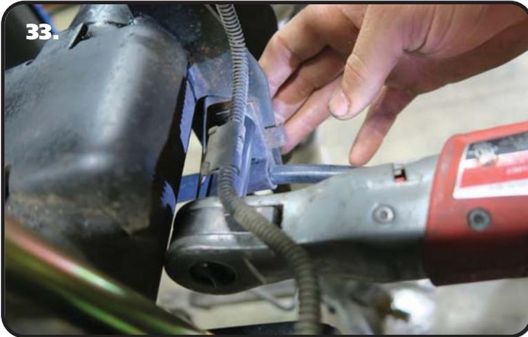
**33.** Unbolt the emergency brake cable clamp from the outside of the driver shock bracket. We will cover reattaching it later in the instructions.
