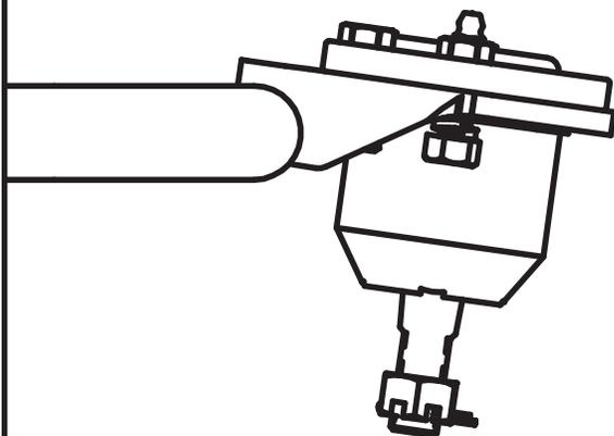
**1.** Remove the Upper Control Arms. The Camber Bolts need to be reinstalled in the same positions they are removed from. We recommend marking their positions for reassembly. Refer to the factory service manual for disassembly procedure. After removing the factory upper control arm, clean the bushing mounting surfaces on the frame.
