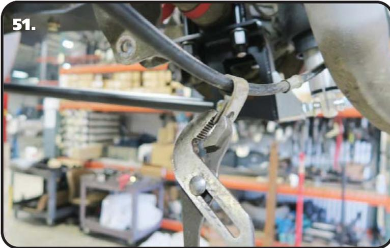
**51.** Reinstall the removed clamp with the ears pointing upward. Install the clamp on the cable and close it with a pair of pliers. Reattach the clamp to the OEM mount using the OEM hardware.
