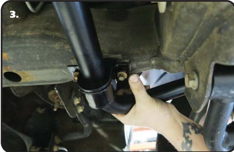
3. Slide the MuscleBar into position on the truck. The SwayBar Arms will be above the steering linkage. Install Bushing Straps Over the Poly MuscleBar Bushing and bolt them in place using the OEM hardware. Do not tighten the hardware until the PosiLinks are hooked up to the MuscleBar.
