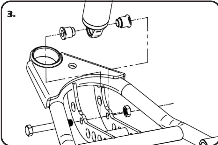
3. Raise the lower arm up to the CoilOver and bolt them together using the 1/2" x 3 1/2" bolt, flat washer, and nylok supplied w/ the lower arms. An aluminum spacer will be on each side of the bearing. Torque to 75 ftlbs.
