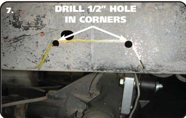
7. Use the supplied Template to mark the cut lines on the frame, then drill out the two corners with a 1/2" drill bit. This will give the cut a round edge and eliminate the possibility for stress fractures. Then cut the notch with a saw-z-all, cutoff wheel, or plasma cutter. Grind all edges smooth. Check the inside of the frame for wires or lines before drilling or cutting.
