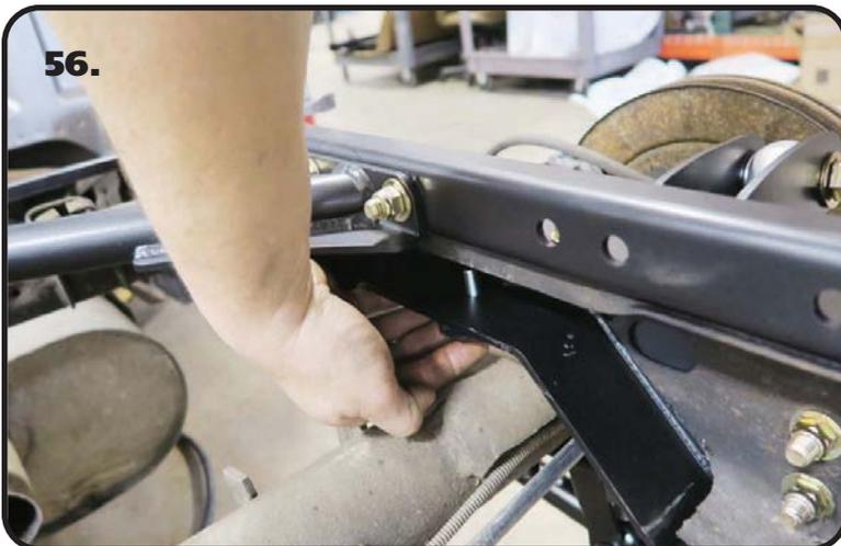
**56.** Install the Bumpstops into the C-Notch above the axle using the 3/8" Flat Washer and 3/8"-16 Nylok Nut supplied. A bumpstop will need to be installed in each c-notch.
