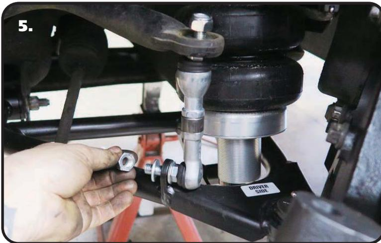
5. Install a 7/16" Flat Washer onto the threads of the 90 Degree PosiLink. Insert the PosiLink into the swaybar tab on the control arm with the threads pointing to the FRONT of the truck. Install a 7/16" Flat Washer and M12 - 1.75 Nylok Nut and torque to 50 ftlbs.
