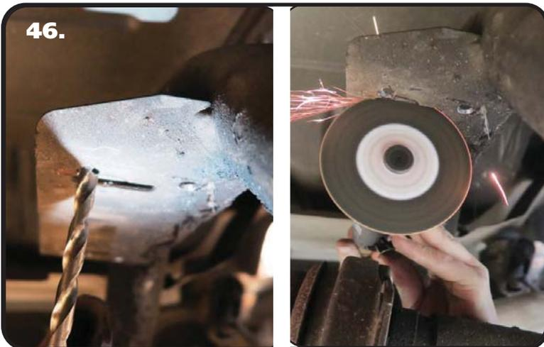
**46.** Image 46 illustrates drilling and cutting the OEM carrier bearing mount. Drill the (4) marked holes using a 3/8" drill bit. Cut along the line that was marked along the inner edge of the new mount. This will remove the center of the OEM mount.
