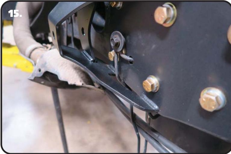
**15.** Reinstall the emergency brake cable bracket using the OEM hardware.
