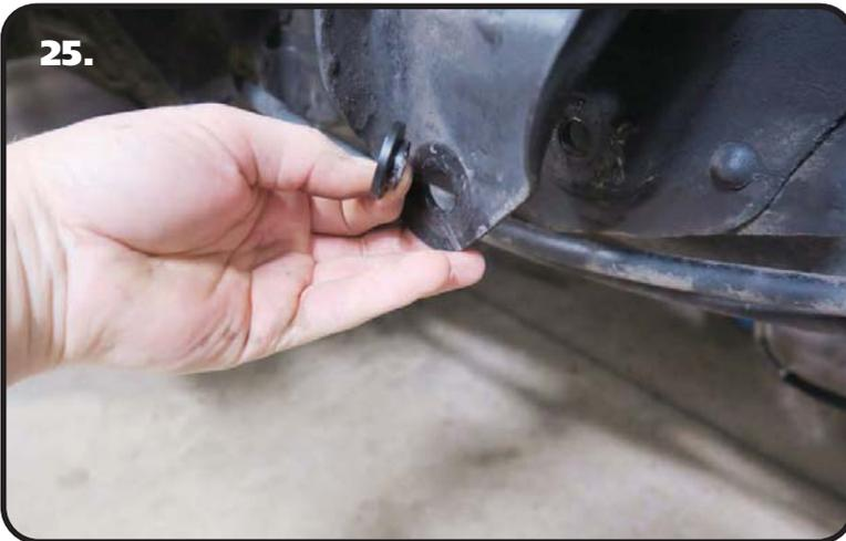
**25.** The kit includes (4) t-busings for the front leaf spring mount. Insert a t-bushing in each front leaf spring mounting hole with the small OD inserted into the hole. The large OD needs to be on the outside of the brackets.
