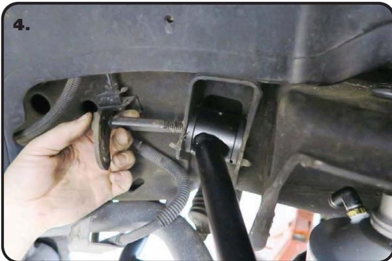
4. Bolt the arm to the frame using the factory camber bolts.
