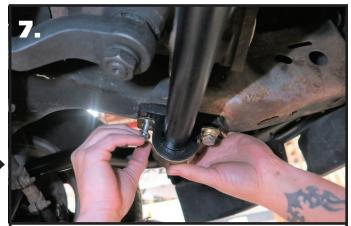
**7.** Slide the SwayBar into position on the truck with the SwayBar arms above the tie rods. Install a Lock Washer & Flat Washer on the each M10 Hex Bolts. A 30mm goes in the front, with a 40mm going in the rear. Do **NOT** complete tighten the hardware at this time.
