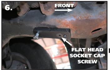
**6.** Hold the Frame Plate up to the OEM holes, the Counter Sunk hole will he positioned over the front hole with the slot to the rear. Apply Red Loctite to the Flat Head Bolt. Thread a Bolt into the rear hole to help keep the plate straight. Torque the flat head bolt and remove the rear bolt.
