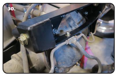
**30.** Using the Hardware Bag "Brake Line Junction Block", install a 5/16" Flat Washer on a 5/16"-18 x 1 1/2" Bolts. Insert the bolt/washer through the junction block and mounting hole in the differential bracket. Install a 5/16" Flat Washer & 5/16"-18 Nylok Nut on the threads of the bolt. The brake lines will need to be tweaked to get the distribution block in position. Torque the bolts to 25 ftlbs.
