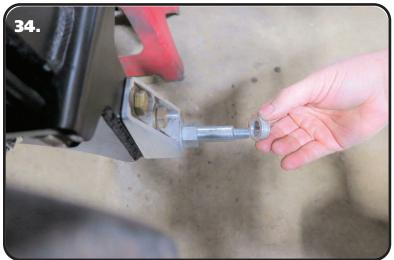
**34.** The Shock Stud requires spacers that are .400" long (90002067). Install a 5/8" ID 90002067 spacer **(Small side towards shock body)** onto the lower Shock Stud. Slide the bottom of the Shock onto the Stud. Install a second 5/8" ID 90002067 Spacer onto the Stud **(small side towards shock)**. You may need to jack the rearend up to Slide the Shock onto the Stud.
