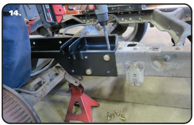
**14.** Use a 7/16" Drill bit to drill the remaining holes in the top and bottom of the frame. Install a 7/16" Flat Washer on the remaining 7/16" x 1 1/4" Bolts. Insert bolt/washers in the drilled holes of the c-notch. Install a 7/16" Flat washer and 7/16" Nylok Nut on the threads sticking through the c-notch/frame.
