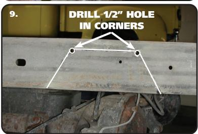
**9.** Drill out the two corners with a ½" drill bit. This will give the cut a round edge and eliminate the possibility for stress fractures. Then cut the notch with a saw-z-all, cutoff wheel, or plasma cutter. Grind all edges smooth. Check the inside of the frame for wires or lines before drilling or cutting.
