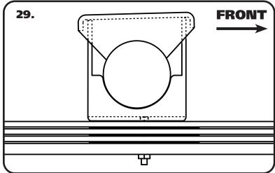
**29.** Slowly lower the axle into the Flip Bracket making sure the tabs go up into the leaf spring saddle.
