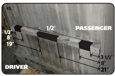
**15.** The bed brace between the wheel wells will need to be trimmed to clear the C-Notches and center section of the axle housing. Use **Image 15** as a reference for cutting. The outer cuts require removing the entire section of the brace. Leave a 1/2" of the brace in the center cut. Reinstall the bed using the OEM hardware.
