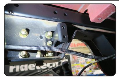
**13.** Slip the Brake Line Bracket over the 7/16" and 5/16" Bolts sticking through the back side of the frame. Install a Flat Washer & Nut on each and tighten.
