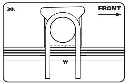
**30.** Slip the U-Bolts over the axle tube with the threads pointing down.
