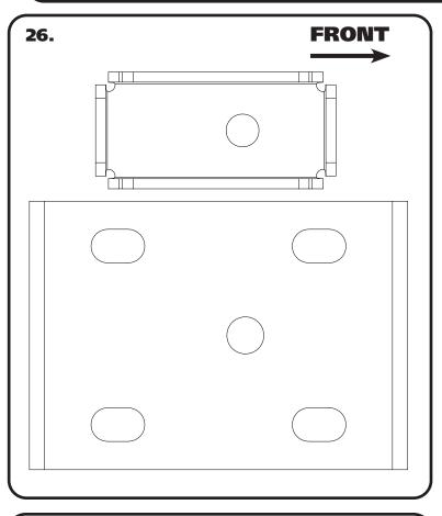
**26.** The Flip Kit has an offset locating holes to center the wheel in the wheel opening. **Image 26** illustrates a top view of the Flip Bracket and the Leaf Spring Plate. Notice the CENTER Hole is offset to the FRONT of the truck. This kit will move the axle rearward.
