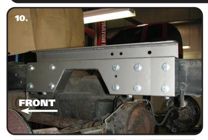
**10.** Slip the C-Notch over the frame rail. Use the C-Notch as a template to drill the (10) holes in the side and (3) in the bottom. Use a 7/16" drill bit to drill the holes. Install a 7/16" Flat Washer on each of (10) 7/16"-14 x 1 1/2" Bolts. Insert a bolt/washer in each hole. Install a 7/16" Flat Washer and 7/16"-14 Nylok Nut on the threads of each bolt/washer and tighten. Torque the hardware to 75 ftlbs.
