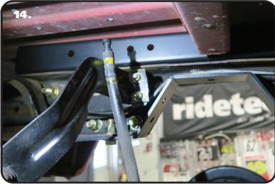
**14.** Install a 5/16" Flat Washer on each of (2) 5/16" x 1 1/4" Bolts. Install them in the Brake Line Bracket and slip the OEM brake line bracket over the (2) bolts. Install a 5/16" Flat washer & 5/16" Nylok Nut on each bolt and tighten.
