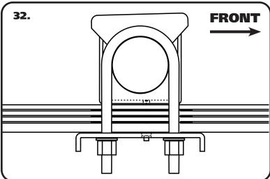
**32.** Hold the Leaf Spring Bracket in place and install (4) 9/16" Flat Washer & (4) 9/16" Hugh Nuts on the threads of the u-bolts. Snug the nuts down evenly and tighten them in a crisscross fashion to 90 ftlbs.
