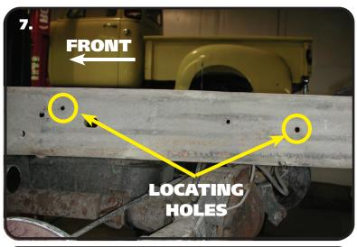
7. To allow maximum drop on this truck, the frame must be notched. The template for the notch will locate off of the 2 existing holes. Image 7 illustrates the holes used. Use the supplied "C" Notch template to mark out the frame for cutting. Before cutting out the frame, support the frame in front of and behind the "C" Notch area. We suggest doing one side at a time.
