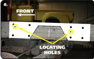
**8.** Use the supplied Template to mark the cut lines on the frame. Center Punch the "\(\psi\)" in the corners of the cut area.
