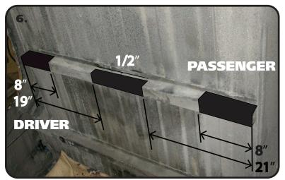
CUTTING THE BED BRACE WITH THE BED INSTALLED. IF REMOVING THE BED, REFER TO STEP 15 FOR BED BRACE CUTTING.
