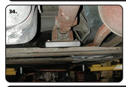
**34.** Install carrier bearing spacer between carrier bearing housing and cross member. Secure with 3/8" x 2 1/2" bolts, 3/8" flat washers, & 3/8" nylok nuts. Torque to 30 ftlbs.
