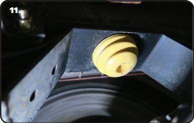
**11.** Bolt the Bumpstop into the C-notch using the hardware included on the bumpstop.
