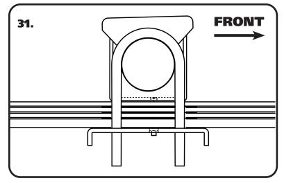
**31.** Slip the Leaf Spring Bracket up onto the U-Bolts WITH THE OFFSET HOLE FORWARD.
