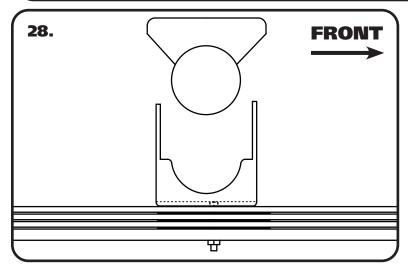
**28.** Set the Flip Bracket onto the leaf spring with the CENTER HOLE OFFSET TO THE FRONT OF THE TRUCK.
