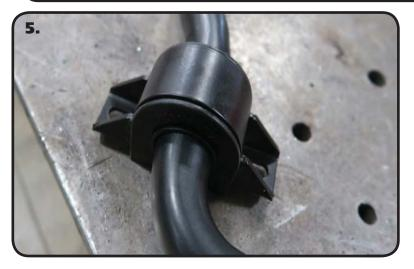
**5.** Install Bushing Straps Over the Poly Sway-Bar Bushings.
