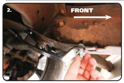
2. The Sway Bar Mount attaches to the frame using the holes from the OEM mount. The end of the frame bracket with the angled bends goes forward. Attach the bracket using a 3/8"-16 x 1 1/4" bolt, 3/8"-16 Nylok nut and a 3/8" Flat Washer on top and bottom. The same harware setup is used in each hole. Repeat on the other side and tighten hardware.
