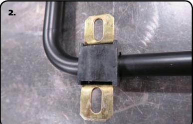
**2.** Open up the Poly SwayBar Bushings and install them over the Delrin Sleeves. Install Bushing Straps Over the Poly SwayBar Bushings.
