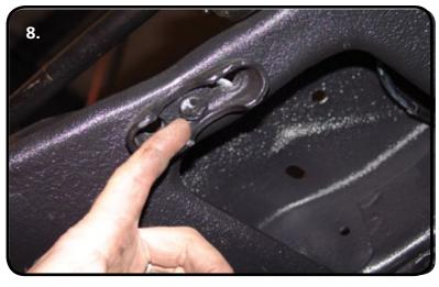
**8.** The lower control arm is installed using the factory U-bolts and nuts. The lower control arm is located by a pin that is in the center of the front u bolt cradle. This pin will go into the hole in the control arm shaft to help locate the control arm.
