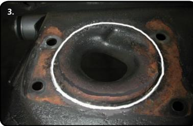
**3.** The top side of the crossmember will also need trimmed for clearance. A TEMPLATE IS PROVIDED ON PAGE 13. Cut out the holes in the template and place on top of the crossmember. Trace the template onto the crossmember and cut out the center portion. Your mark should look similar to the one pictured.
